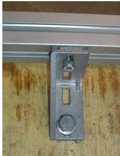
Figur 3 Transport safety for worktable
