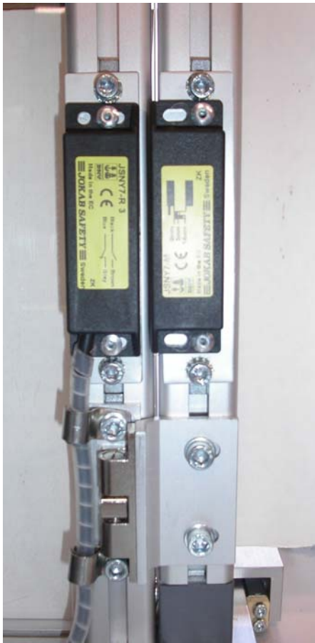
Figure 5 Magnetic switch on Db-Enclosure
